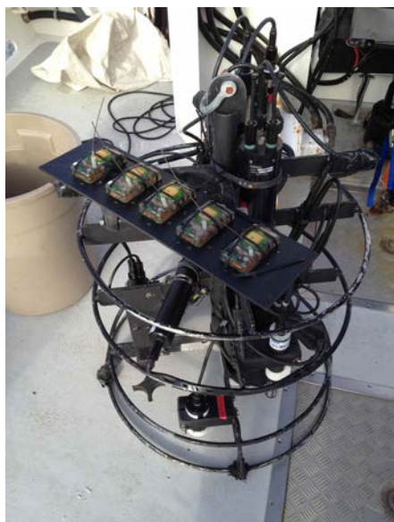
Figure 16: Sampling rosette with temperature, pressure and irradiance sensors and 5 seal tags mounted on a board.
