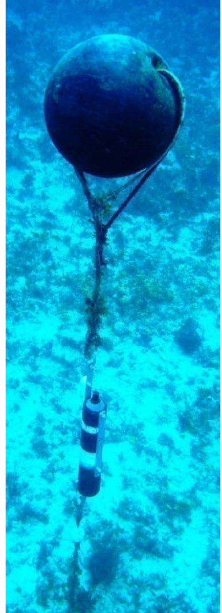
Figure 5: Illustrations of mooring type for VR2W-69; (i) VR2W attached to metal rod with no float (for offshore deployments) and using rock anchor, (ii) VR2W-69 attached to metal rod with cables from anchor to rod and rod to float (potential for Dunganab), and (iii) Auger or sand anchor for Dunganab Bay attachment to substratum.
