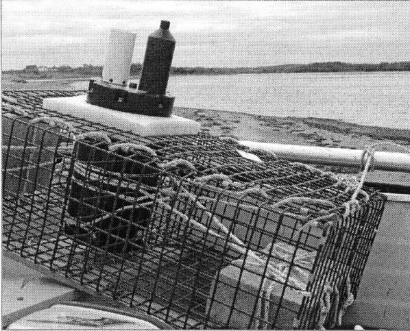
Fig 2. A VR3 receiver mounted in a lobster trap before deployment in Pomquet Harbour channel (SW12 PH; Apr'10).
